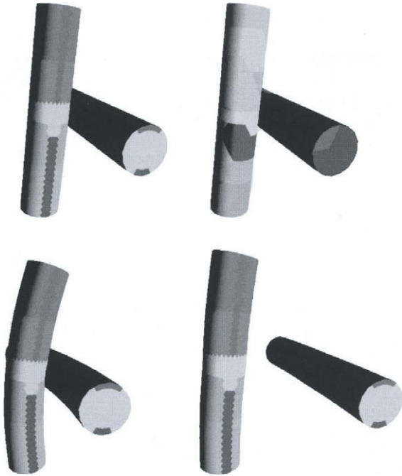
Fig. 2. Impact of two solid cylinders: contact partitioning (top left); solid partitioning (top right); deformed configurations.
