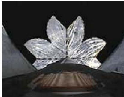
**Figure 7. JAXA deploying a clover shaped solar sail in August 2004**
