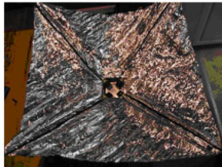
**Figure 5.** 0.58 m<sup>2</sup> drag sail deployment prototype made from a mylar survival blanket. Stowed volume: 5 × 10 × 10 cm<sup>3</sup>
