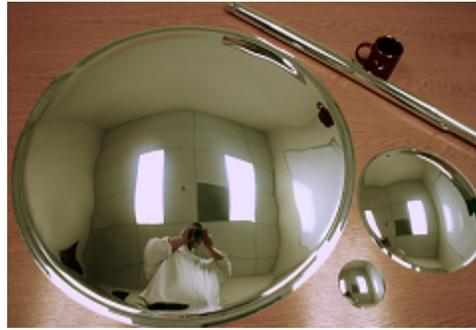
**Figure 6. Mevicon's thin film shells are self supporting in 1 g and roll into thin cylinders for compact stowage.**
