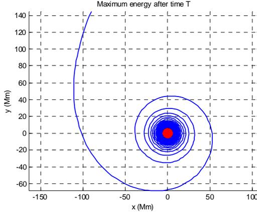
Figure 3. Optimal thrust control of spacecraft to reach escape velocity. Constant thrust ion engine powers spacecraft to maximize orbital energy after time  $T$ . Related problems that can be solved using Pontryagin's Maximum Principle are minimum time to escape velocity, minimum fuel to escape, and minimum constant thrust to escape in time  $T$ .
