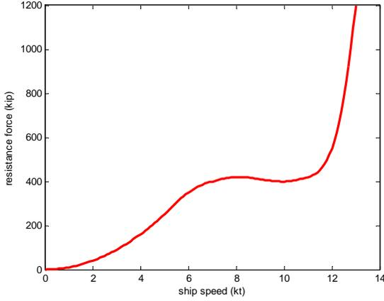
Figure 5. Total hull resistance (thrusting) as function of ship speed. At slow speeds, it can be modeled as viscous friction, proportional to the square of ship speed.
