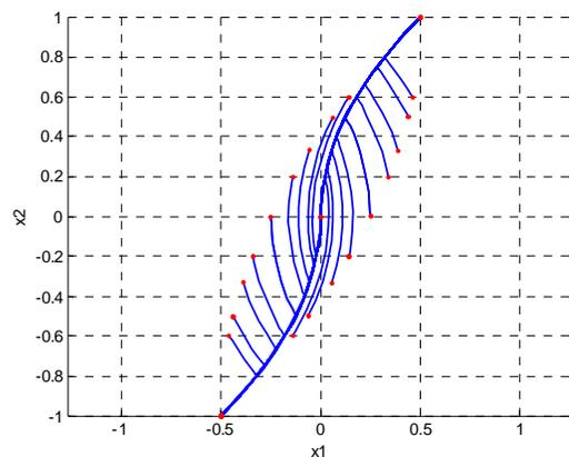
Figure 2. Time optimal control of a double integrator. Phase plane shows optimal trajectory,  $x_1$  is position and  $x_2$  is velocity. The red dots represent various initial conditions. The optimal control is  $u_{\max}$  until reaching switching curve, then it jumps to  $u_{\min}$  driving the state to the origin in minimum time. Pontryagin formalized the theory behind bang-bang control, and extended it to many other important problems.
